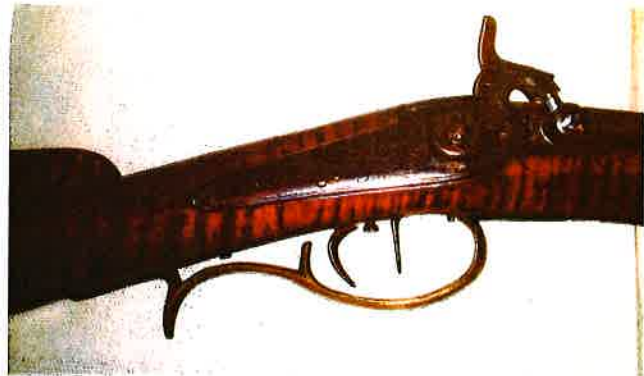
Fig. 2. Back action lock area and trigger guard of a H. Burns rifle once owned by the author's father.
