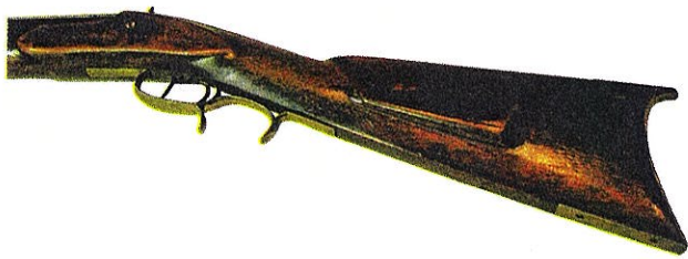
Cheekpiece side view of Samuel Hawken rifle. Note rectangular cheekpiece, brass trigger guard traditionally mounted to stock, and flat-end toe piece. Held by Cody Firearms Museum 1997.4.5. Gift of William B. Ruger and Sturm, Ruger. (Photograph by Nathan E. Bender)
