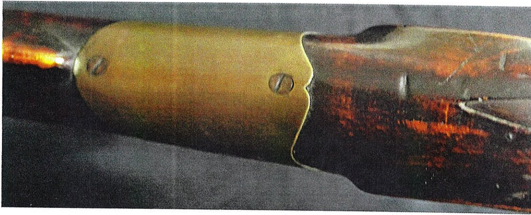
Fig. 3. Brass wrist repair (lock side view).
