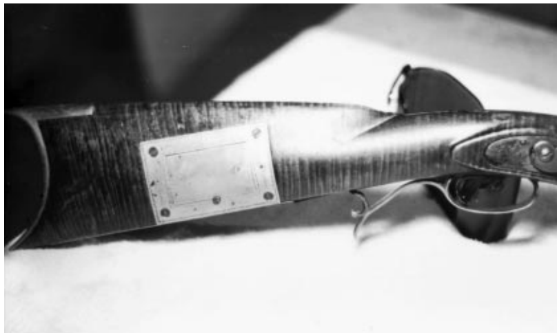
Illustration No. 6a: Patchbox side of a later Indiana fullstock rifle, ca. 1860's, by Wareham. Note the "Indiana style" trigger guard with drooping rear spur. Wareham used his characteristic wavy border engraving on the little patchbox, and low comb line. The exceptionally fine curly maple is unexpected for a later rifle. The gun came out of a family in Waterloo, Indiana where Wareham worked. Photo by Author.
